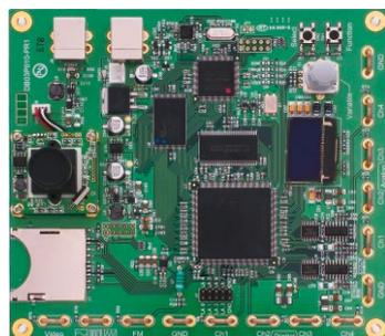
The GDB-03 training kit allows you to learn both the basic and the advanced functions of the GDS-3000 Series, GDS-2000A Series/GDS-2000E Series/MSO-2000 Series and GDS-1000B Series Digital Storage Oscilloscope (DSO). Following the training procedures of this training kit, you will quickly understand the basic operations of a DSO, and the unique features, which represents a typical hi-tech DSO today.
